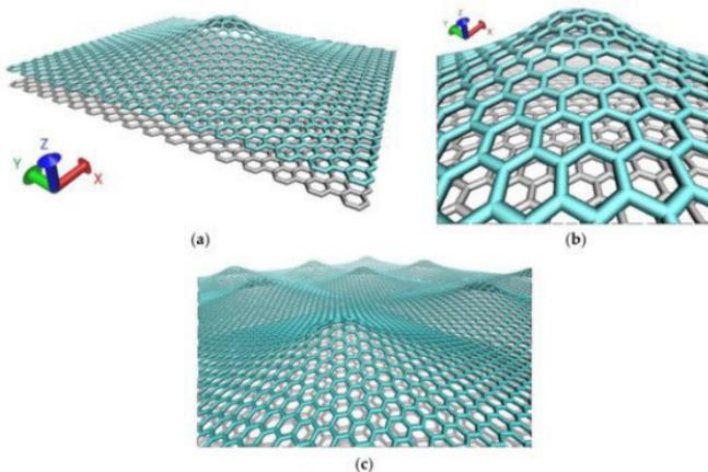
**Figure 1:** Atomic model of graphene nanoblister: (a) super-cell; (b) the tip of the nanoblister; (c) the overview of the nanoblister surface (the substrate is noted by silver color, the monolayer with graphene nanoblisters is noted by blue color).
