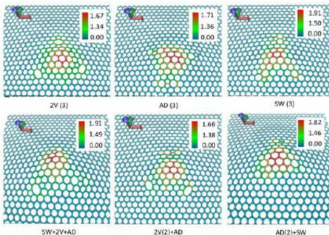
**Figure 2:** Maps of the local atomic stress of investigated graphene nanoblister for various defects. A calibration scale of stresses in GPa is indicated in the top right corner of each picture.
